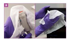
Use the wipe to disinfect the skin surface probe. Another wipe can be used for the monitor, keyboard, probe holders and cables.
